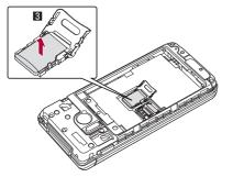
3 Close the microSD card slot cover (4) and slide locked (5)
